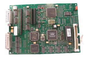
Modular design plug-in circuit board. Offers programmable FLASH memory for easy firmware upgrades. Includes a 20,000-event history buffer and a computer micro-processor. Performs Internet and intranet alarm monitoring and operates as a 32 telephone line digital receiver.
